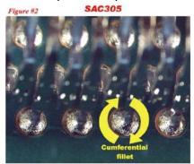
Source CE Analytics; Both through-hole connections exhibited good solder filet and circumferential wetting present on secondary source side of the solder joint coated with OSP. The SACX0307 exhibited a slightly better circumferential wetting
